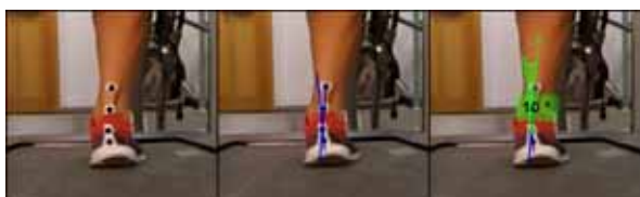
Figure 1. Markers placed on the right lower limb of a participant, lines representing the long axis of the rearfoot and the shank, and peak eversion angle measured with Kinovea software.
