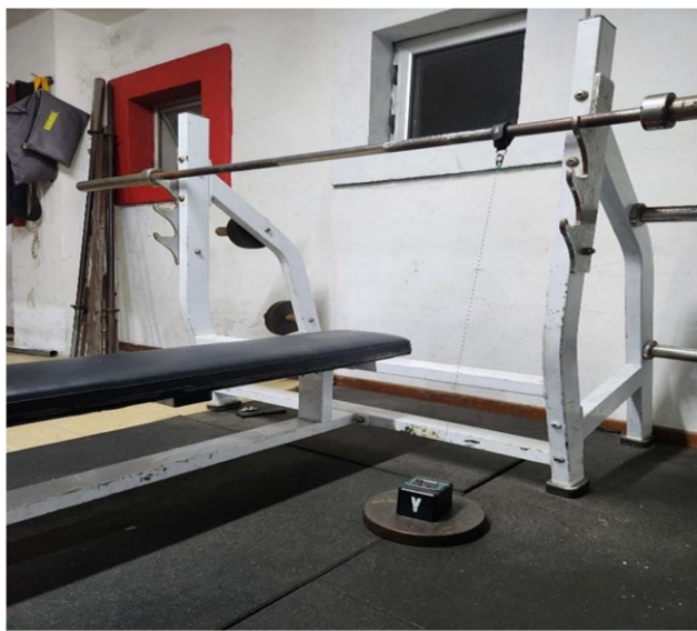
Figure 1. Flat bench, barbell and linear Encoder used to perform the maximum voluntary repetition (1MR) test in the bench press exercise
