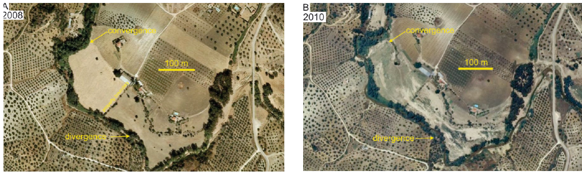
Figure 6. A. GeoMap image from 2008 showing the area before the flooding events. B. GeoMap image from 2010 showing the area following earthworks on the floodplain and at the divergence point. The remnants of the downstream end of the avulsion channel can be seen leading to the convergence point. Cropping on the floodplain resumed after this date.
