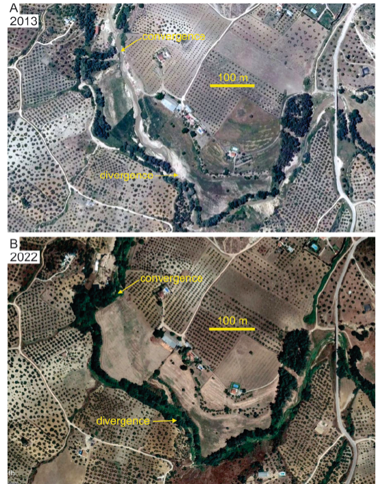
Figure 9. A. GeaMap image showing the avulsion channel in mid-2013. Note the light-coloured flood sediments along the old irrigation channel. B. Google Earth image from 2022. The downstream property has been levelled, the levee at the divergence point has been repaired and the river has been returned to its former location. The avulsion channel fill shows as slightly darker tones. The avulsion channel on the upstream property is lined with low trees but has not been levelled.
