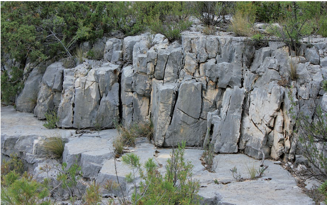
Figura 4. Capa de calizas micríticas, afectada por un sistema subvertical de diaclasas, que no se continúan en el estrato inferior. Figure 4. Layer of limestones, affected by vertical joints which are not continued in the lower bed.
