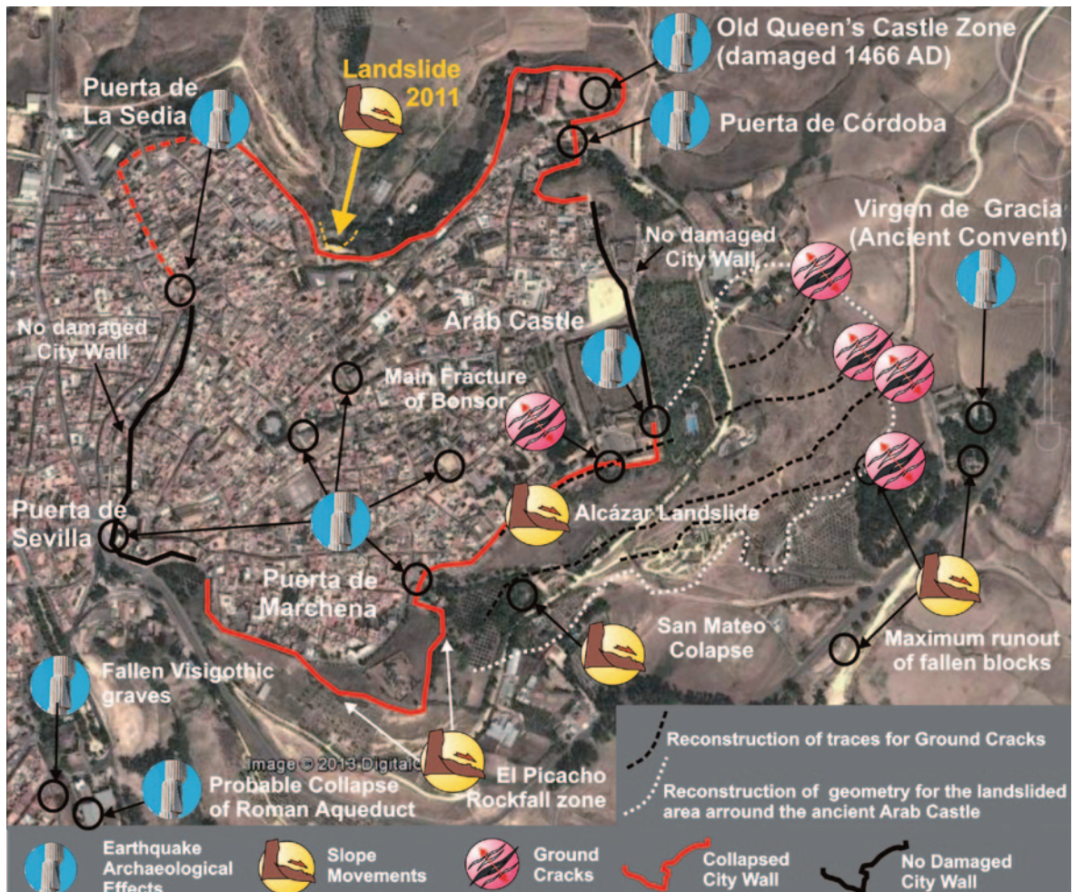
Figure 3. Aerial plan-view (Goggle Earth) of the Carmona city displaying the ground cracks documented by Bonsor (1918) affecting the ancient Arab Castle (Alcázar) walls and the Virgen de Gracia Church (Ancient Los Jerónimos Convent) in the context of the area that underwent landsliding. The sector of the ancient city walls (north and south) damaged by the earthquake are highlighted in red, as well as different documented archaeoseismological effects cited by Bonsor (1918) around Carmona. The recent building constructed on the ancient damaged ruins of the Castle is the Parador Nacional de Turismo de Carmona (1976).
